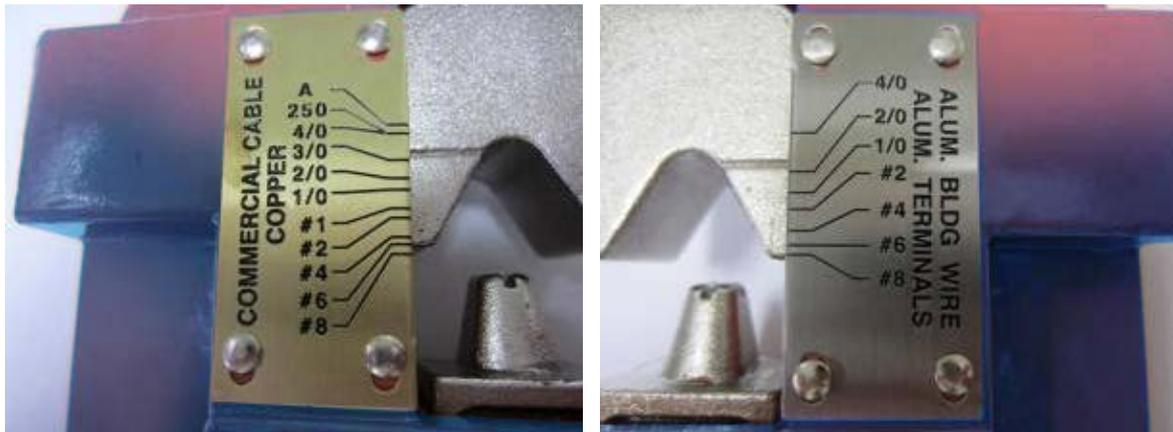
3. Due to different brands of terminals and cables, there will be slight size difference. For the first time use, please adjust the scale on V shape part to be between the size of terminal needs to be crimped and one size bigger. For example, if you'd like to crimp 3/0 terminal, please adjust the scale to be between 3/0 and 4/0 for the first time to find out the best position of crimping. The position of scale can be adjusted in anti-clockwise direction of the black knob on the top.
