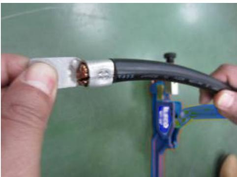
8. If the terminal was not crimped tightly enough, adjust the V shape part to be tighter by adjusting the black knob in clockwise direction until it can crimp the terminal properly. Then keep the position for next crimping job.
