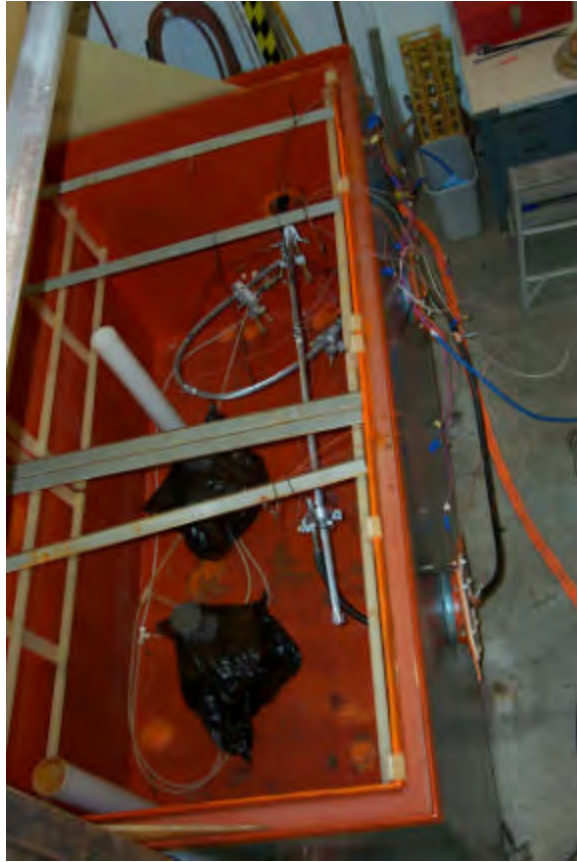
Photograph 3 Salt Fog Chamber with Connector Loop
