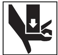
**Keep your fingers and hands away from the interchangeable head during the operating cycle. Your fingers or hands can be crushed, fractured or amputated in the interchangeable head or tool or between the interchangeable head, work piece and other objects.**
